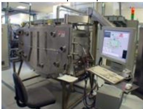
Figure 9 - Reel-to-reel vacuum deposition line.
