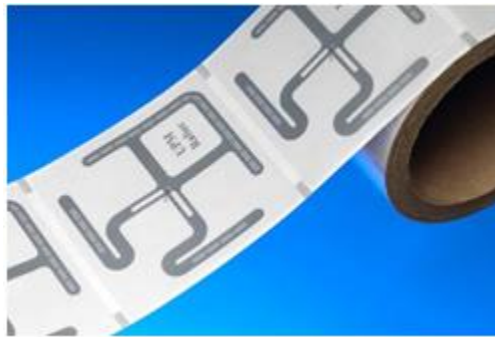
Figure 12 - Silicon Radio Frequency Identification (RFID) chip with antenna processed using R2R technology [20].
