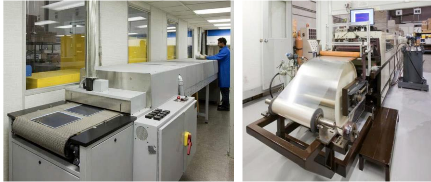
Figure 7 - (Left) screen printing and (right) tape casting. Photos from M. Richards, Versa Power Systems
